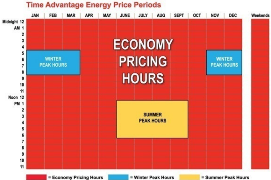
Figure 6 - TOU Hours This diagram show the times of day and months of the year where peak pricing is used in Alabama Power's Time Advantage (a.k.a. TOU) rate offering [35] .
